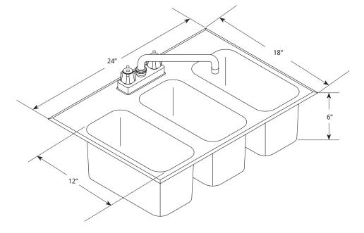
Note: For counter cut out, subtract 1" from length and depth dimensions.
