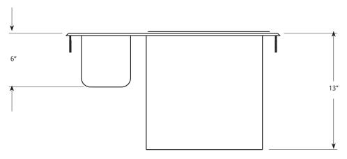
Note: For counter cut out, subtract 2 5/8" from length and depth dimensions.
